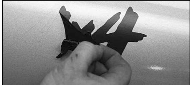
Figure 6 The time required to cleanly remove a vinyl graphic of this size can be performed in a matter of seconds using the fast-off pad.
