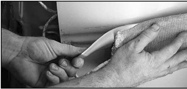
Figure 5 This side moulding was removed in several minutes. Wider or thicker mouldings may require more time.
