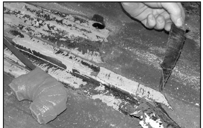
Figure 4 The Glass Blaster attachment is being used to remove sprayed-on bed liner material.
