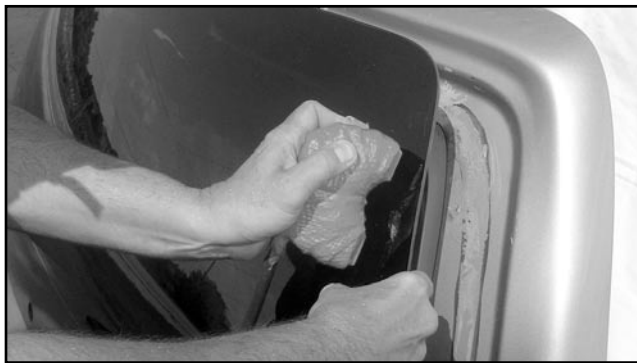
Figure 3 As shown here, the urethane adhesive will remain attached to the glass with little or no clean up of the pinch weld needed. Glass to be reinstalled will require clean up.
